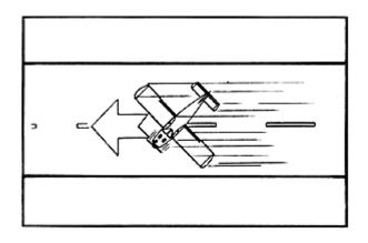
Skidding sideways is a fast ticket to blown tires or collapsed landing gear.
