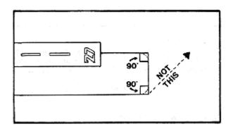
As another aid, set the heading bug on the DG (or heading indicator) if so equipped. The "bug" helps in flying a square pattern at night.
