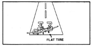
If a nosewheel is flat or the nose gear won't extend, you may want to carefully shift weight aft (within limits, of course) to help hold the nose *off* the runway until the aircraft slows. Passengers can move to rear seats if these seats are empty!
