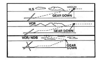
The second "school" suggests extending the gear on downwind, abeam the runway, if the runway is in sight. The advantage of this second technique is that if you lose the runway, a go-around is easier without the gear already being down. The disadvantage is that it's non-standard from your straight-in habit pattern and may cause a distraction when you are trying to keep the runway in sight. You may forget the gear. That's why a last gear check on short final is strongly advisable.
