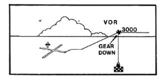
With no final approach fix, extend the gear when you roll out of the procedure turn and start your final descent.
