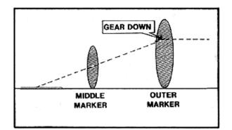
For localizer and VOR approaches. the gear should be extended when passing the final approach fix (FAF) inbound.
