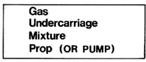
When lowering the gear, always check the gear indicator for "down and locked." Make it a habit to physically touch the gear indicators and say out loud "gear down", or "down and locked," or "three in the green."
