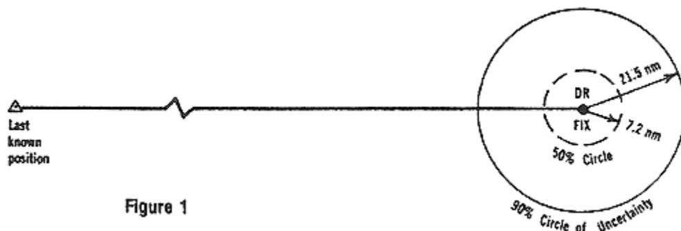
Figure 1, for example, shows where the pilot of a 150-knot aircraft has computed his position to be at the end of one hour. The radius of the circle of uncertainty is equal, therefore, to 20 nautical miles (nm) +1% of which equals 21.5 nm. In other words, there is a 90% probability that the pilot is actually within 21.5 nm of where he thinks he is.
